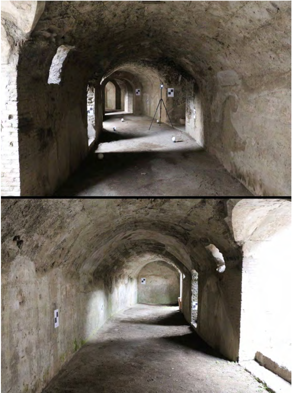
Image 2_Pompeii Amphitheatre: underground ambulatory during 3D laser scanning activities and topographical survey by total station.
